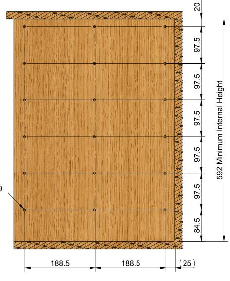
Section view showing machining detail for location hole centres.
