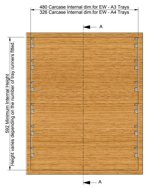
Front View of Carcase with G & T Structural Tray runners in place
